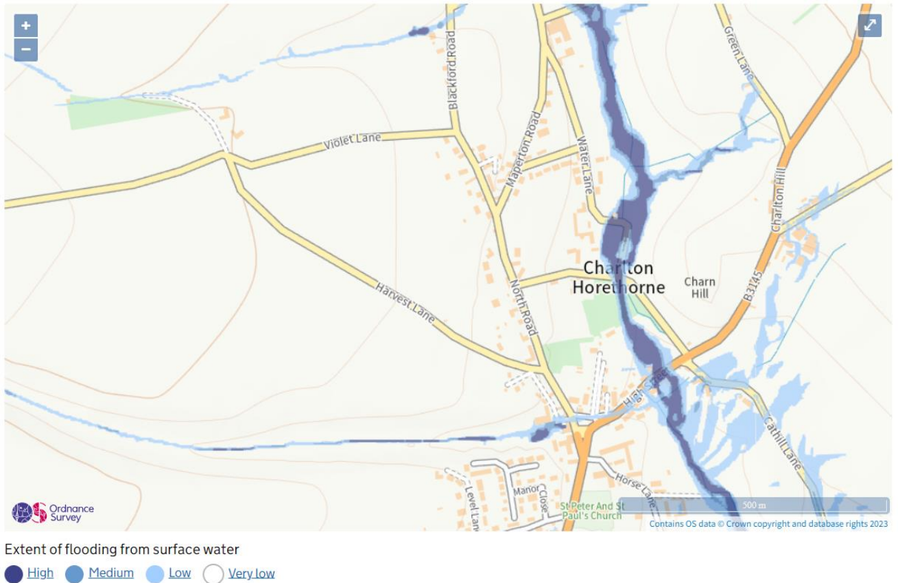
Figure 3: Extent of Flooding from Surface Water Map
